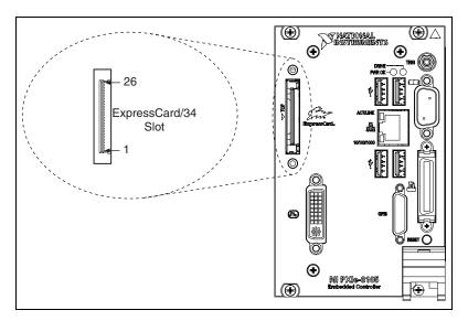
Figure 3-9. ExpressCard/34 Slot Location and Pinout
